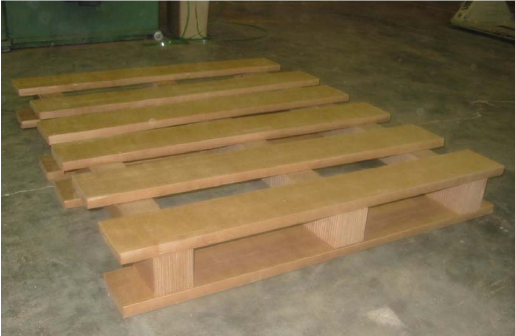
Figure 1: Prototype Paper Engineering 48x40-inch, non-reversible, partial 4-way, stringer style, double wing, corrugated paper pallet.
