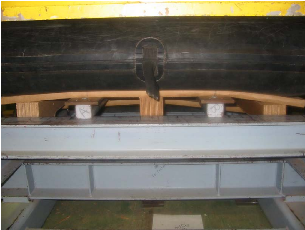
Figure 2: Photograph of the Fork Tine Test Setup. This pallet has been tested to failure.
