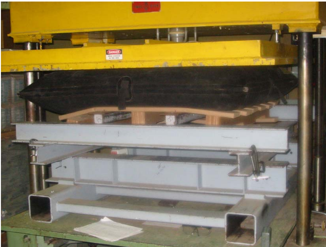
Figure 4: Fork tine support test showing the condition of pallets after testing to failure.
